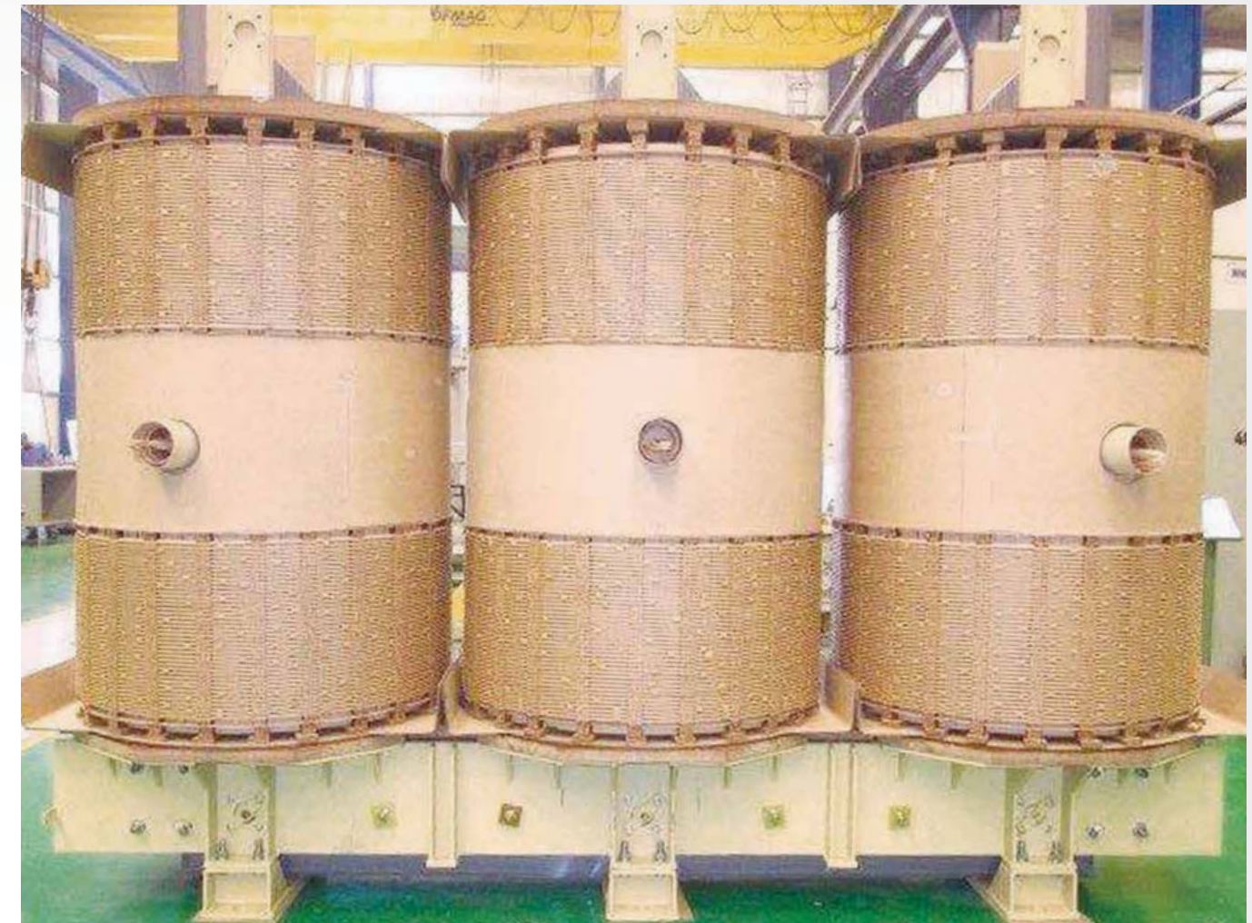
Active part of power transformer 230KV class
