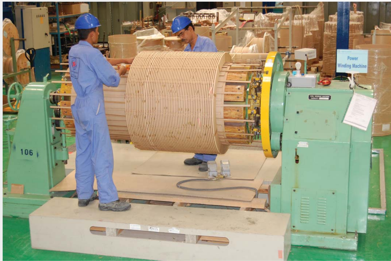
Power transformer winding
